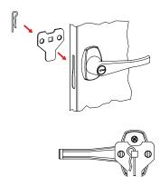
With the handle still in the open position, hook the locking bars (Ref. No. 8) to the locking cam (see "A" at left). Once in position, slowly rotate the door handle to the closed position so the lock bars prot rude from the holes at the top and bottom of the door (shown at right, below).
