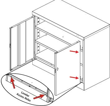
**12.** The cabinet must be level in order for the doors to close properly. Levelers may be adjusted by placing the nut driver through the hole in each end of the sill and adjusting the leveling screw.
