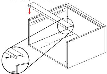
**7.** Place the rear flange of the bottom (Ref. No. 6) into the bottom lances of the back. The flange with two holes should face the front, hanging over the sill. Insert bolts through the bottom and sill with the head facing the front of the unit. Secure with two nuts.
