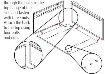
**5.** Attach the right side (Ref. No. 3) to the back in the same manner as you did in step 3, again making sure that the flange is around the back and that the lances on the shelf adjustment strips are pointed in the same direction as those on the back and left side. Push the side panel up so the study in the top.
