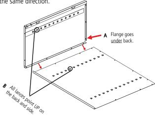
**4.** Attach the top (Ref. No. 7) to the unit by sliding the outer flange over the back of the unit and the side flange to the side panel on the unit. The threaded studs should go
